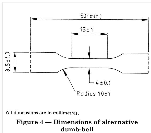
**NOTE** This test piece is particularly suitable for testing seals that are too small to provide test pieces in accordance with type 2 of BS 903-A2 but its use is not restricted to the testing of such, seals.
